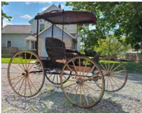
Top Buggy - original condition, Jenny Lind style fringe top with rollup side curtains
