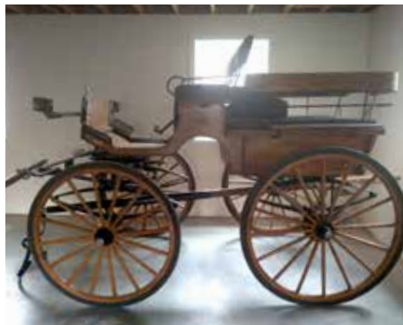
6-Seater Wagon - double hitch pole, single shafts, metal rims
