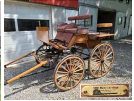
Wagonette/Presentation Carriage - Nice condition, built by Mill Run Carriage, full cut-under, pole and shafts, natural wood finish, tufted Bedford cord upholstery, hydraulic brakes
